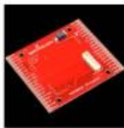
Figure 14 - ADH8066 breakout board
